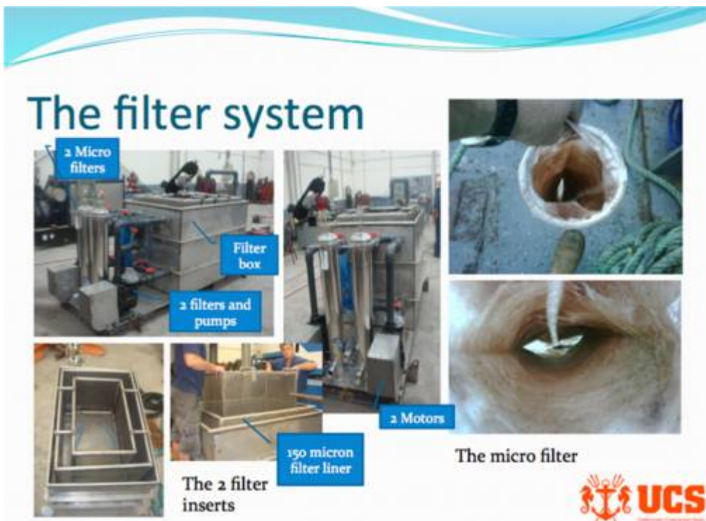
Figure 5. Above, the complete Trident V system. Figure 6. Below, details of the filter system, which makes use of the large surface area of the filter box to remove larger particles. Photos: UCS.
