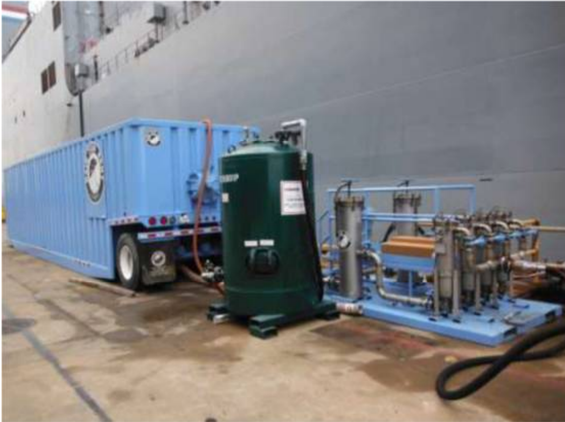
Figure 1. Above, the MARAD/Terraphase scrubber with skirt and propeller-generated suction (center of device), fitted with a hose to capture wastewater, bottom and top views, and below, the pierside debris containment and filter system. Photos from Terraphase Engineering.
