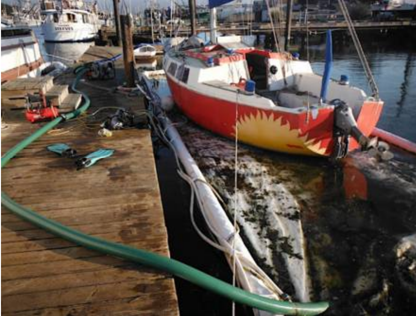
Figure 8. Debris and wastewater being suctioned out of the container following work on a boat. Photos from Innermost Containment Systems.
