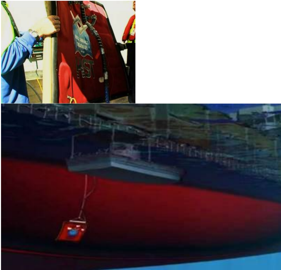
Fig 12. HST’s thermal applicator (shown above) moves along a ship’s hull in a grid pattern, sterilizing the surface. Photos: Leach 2011 and T&C Marine.
