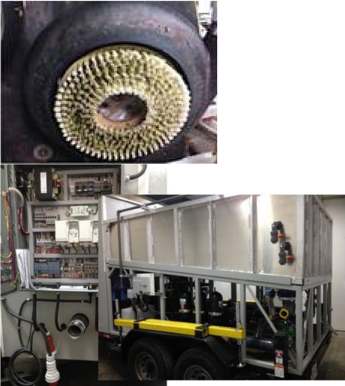
Figure 2. Whale Shark Environmental Technologies rotating brush and filtration system. Photos: All-Sea Enterprises.
