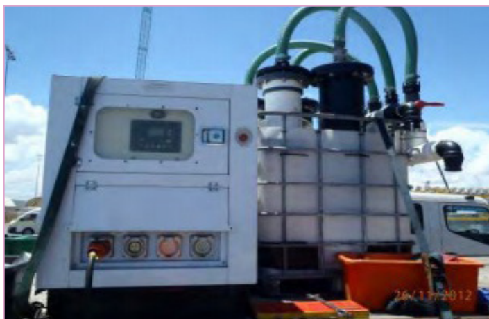
Full-capture in-water cleaning systems capture the water and materials removed from hulls during cleaning. One example is the Envirocart system which has a separate unit (pictured above) that filters and UV treats the water and materials shaved and suctioned off hulls by an attached in-water unit. Source: http://www.fish.wa.gov.au/Documents/occasional_publications/fop114.pdf
