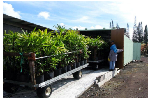
The development and testing of hot water shower boxes like this drive through model is an example of Dr. Hara's work to prevent pest movement in nursery materials.
